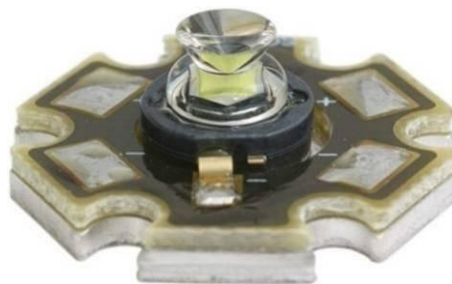
LED modul Luxeon 5W V_f 6,84 V / I_f 700 mA / 5 500 K
