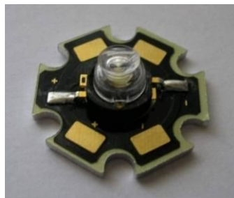
LED modul Luxeon 1W V_f 3,42 V / I_f 350 mA / 5 500 K
