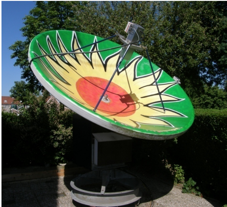
3m Prime focus antenna – PA0PLY
