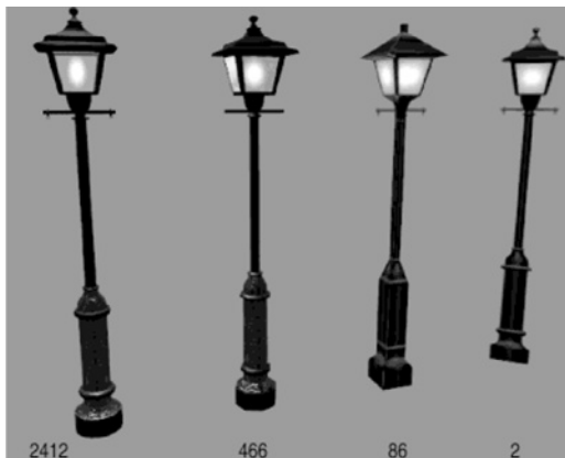
Figure 1-10. LOD example showing poly count of the different versions of an object
