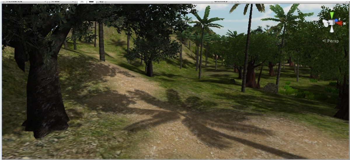
Figure 4-61. Terrain using Pro's dual lightmap system: the foreground shows dynamic shadows plus ambient lightmap; the middle ground and background use full lightmap
