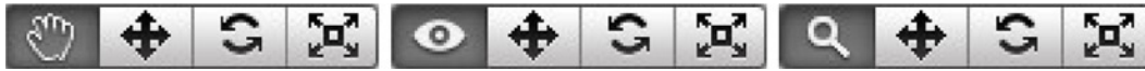
Figure 2-15. Scene navigation tools, pan, orbit, and zoom, (far left of each of the transform buttons)
