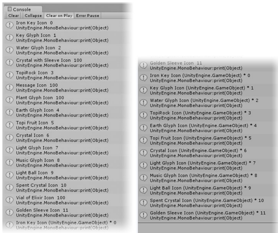
Figure 14-6. The tagged inventory objects and their newly assigned element numbers (left), and the contents of the newly generated currentInventoryObjects array (right)
