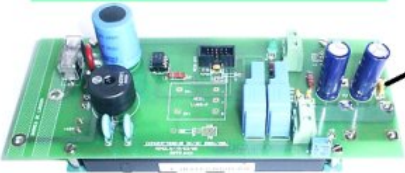
600 W, 300 Vdc / 30 Vdc converter
