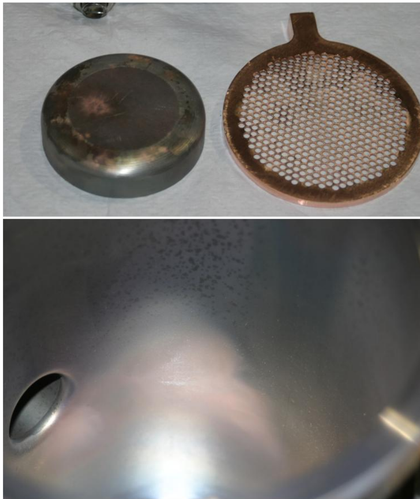
Figure 4.43: Copper deposits on the cathode and SS tube
