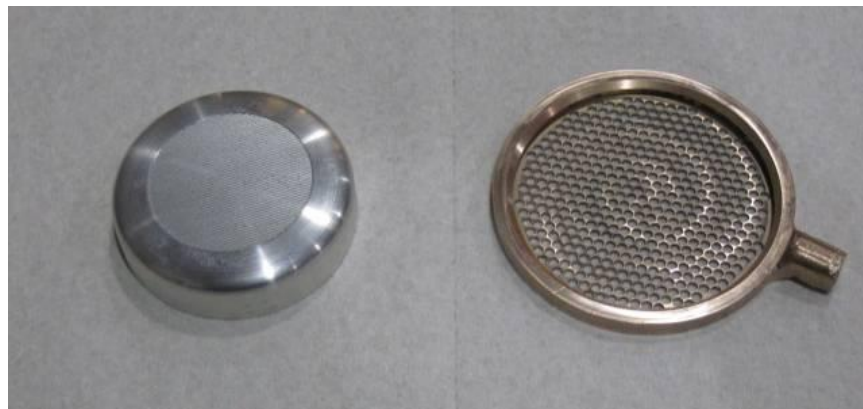
Figure 3.5: Machined aluminum cathode and copper tungsten anode
