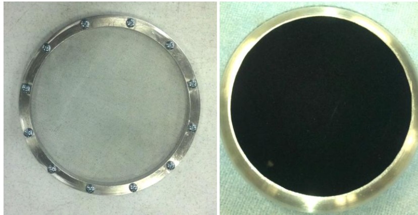
Figure 5.29—Anode screen with holder (left), cathode with black felt emitter (right)
