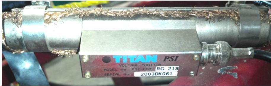
Figure 6.3—Mounted capacitive cable probe
