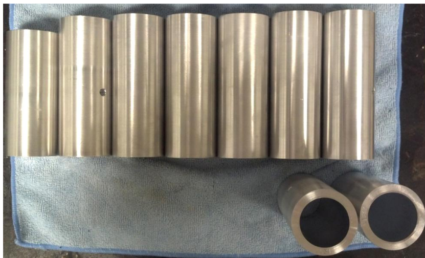
Figure 5.30—Aluminum sleeves used for setting AK gap
