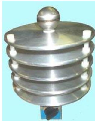
Figure 6.4—Megaprobe from North Star High Voltage [6]
