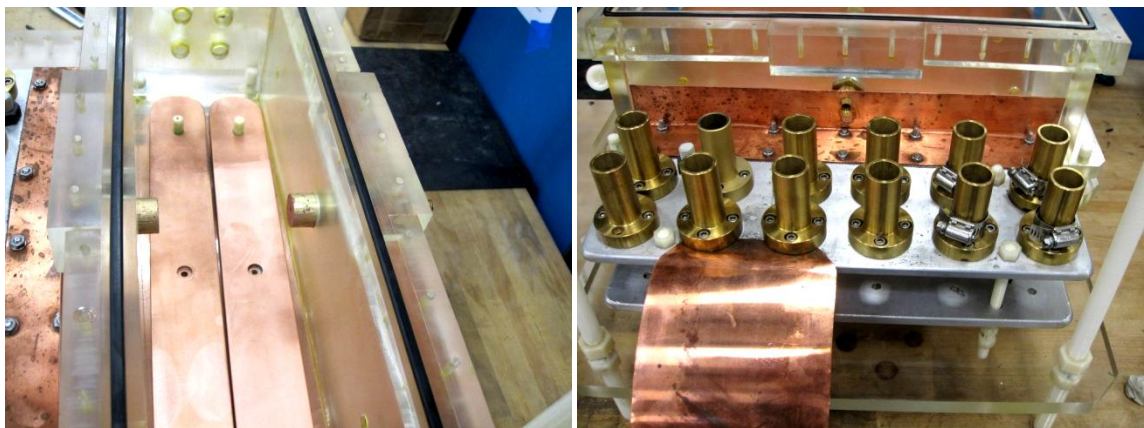
Figure 3.21—Pulse generator load resistor before assembly
