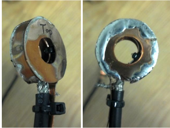
Figure 6.5—Multi-view of B-dot current monitor
