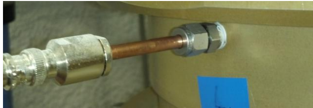
Figure 6.2—Mounted D-dot probe
