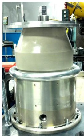
Figure 3.14—High pressure oil switch
