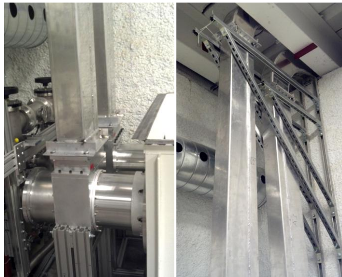
Figure 5.27—Dual vircators connected to output waveguides
