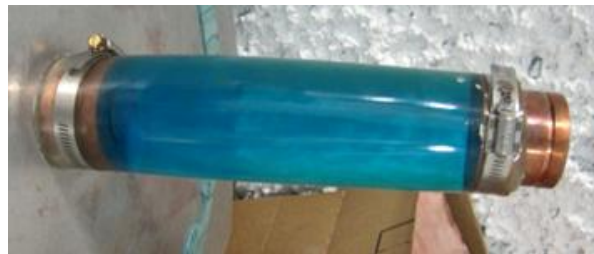
Figure 3.22—Single high voltage load resistor for adder output
