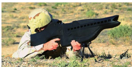
Obr. 5. PHaSR - Personnel Halting and Stimulation Response [7]
