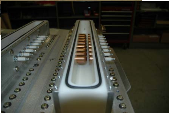
700 kA sparkgap switch
