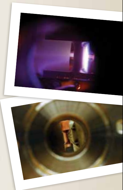
Top: Ions in the Rutgers cyclotron spiral down during a test run. Photo: Tim Koeth
