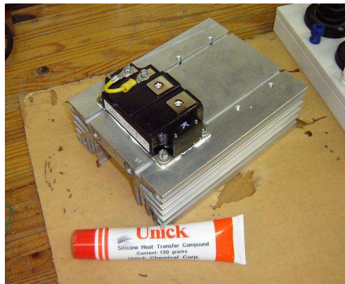
Figure 30: The Mitsubishi IGBT securely mounted onto heat-sink and heat transfer paste used.
