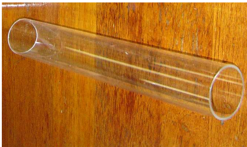
Figure 24: Clear Perspex tubing (50mm Outer Diameter and a 2mm wall thickness) used in the construction of the laboratory scale test launcher.
