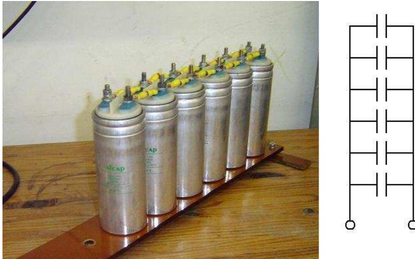
Figure 96: Actual capacitor bank used in laboratory test launcher (Left) and schematic representation of this bank(Right).
