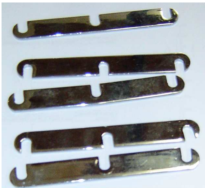
Figure 32: Nickel plated copper motor connection bars which replaced crimped capacitor connectors as shown in Figure 31.
