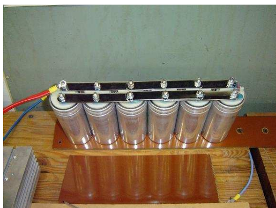
Figure 32: Nickel plated copper motor connection bars which replaced crimped capacitor connectors as shown in Figure 31.
