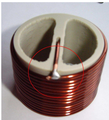
Figure 21: Close up view of the solder joint implementation, the exposed copper wire can be seen on the wire which emerges from the coils center. Also reflected quite well in this figure is the wire location groove.
