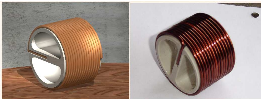
Figure 20: ProEngineer 3D rendering of the armature coil on the left, while the actual armature coil before varnishing is shown on the right. This figure illustrates many details of the armature coil form and the similarity between design concept and implementation.
