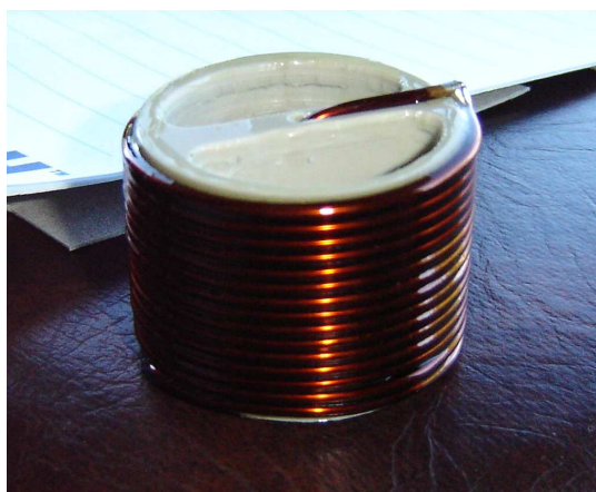
Figure 22: Close up view of an armature coil complete after being coated in 6 coats of varnish.
