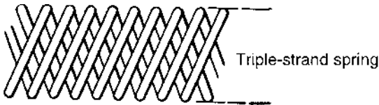
Fig. 8 This flexible shaft permits any shaft angle. These shafts, if long, should be supported to prevent backlash and coiling.
