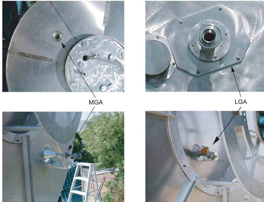
Fig. 4-25. Mars Exploration Rover MGA and LGA mounted on the cruise-stage mock-up.
