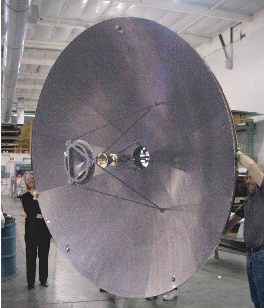
Fig. 4-39. Mars Reconnaissance Orbiter HGA and its X-/Ka-band feed.
