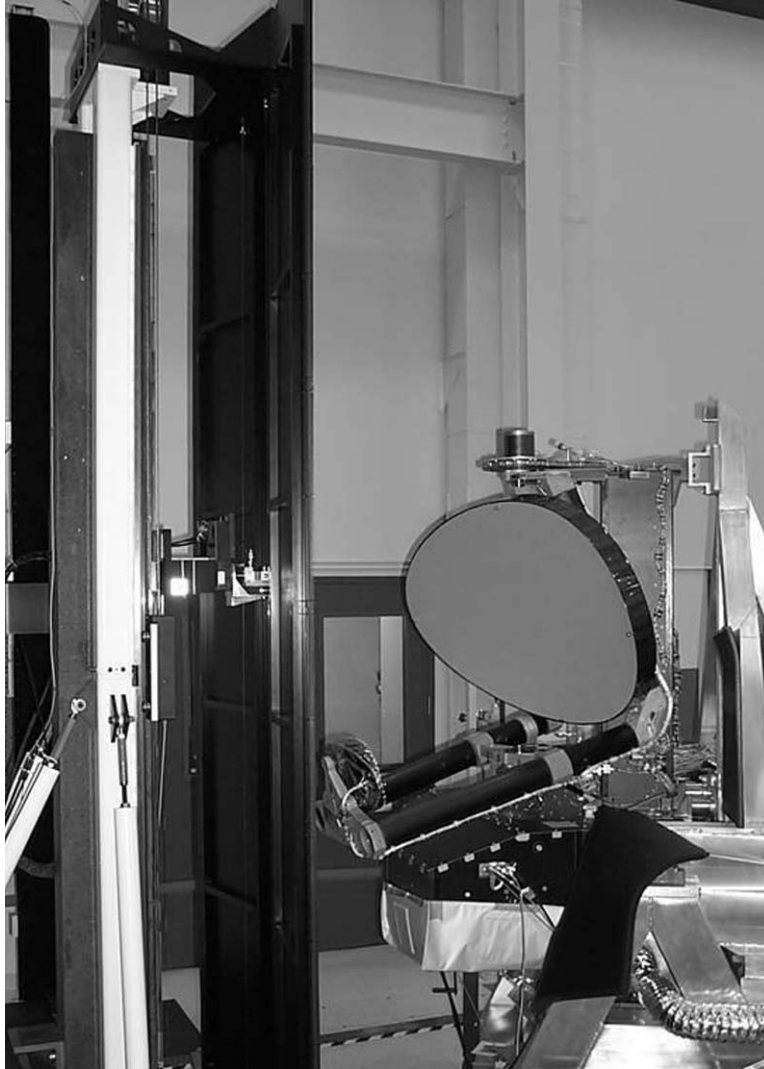
Fig. 7-13. EOS MLS GHz module on near-field range.
