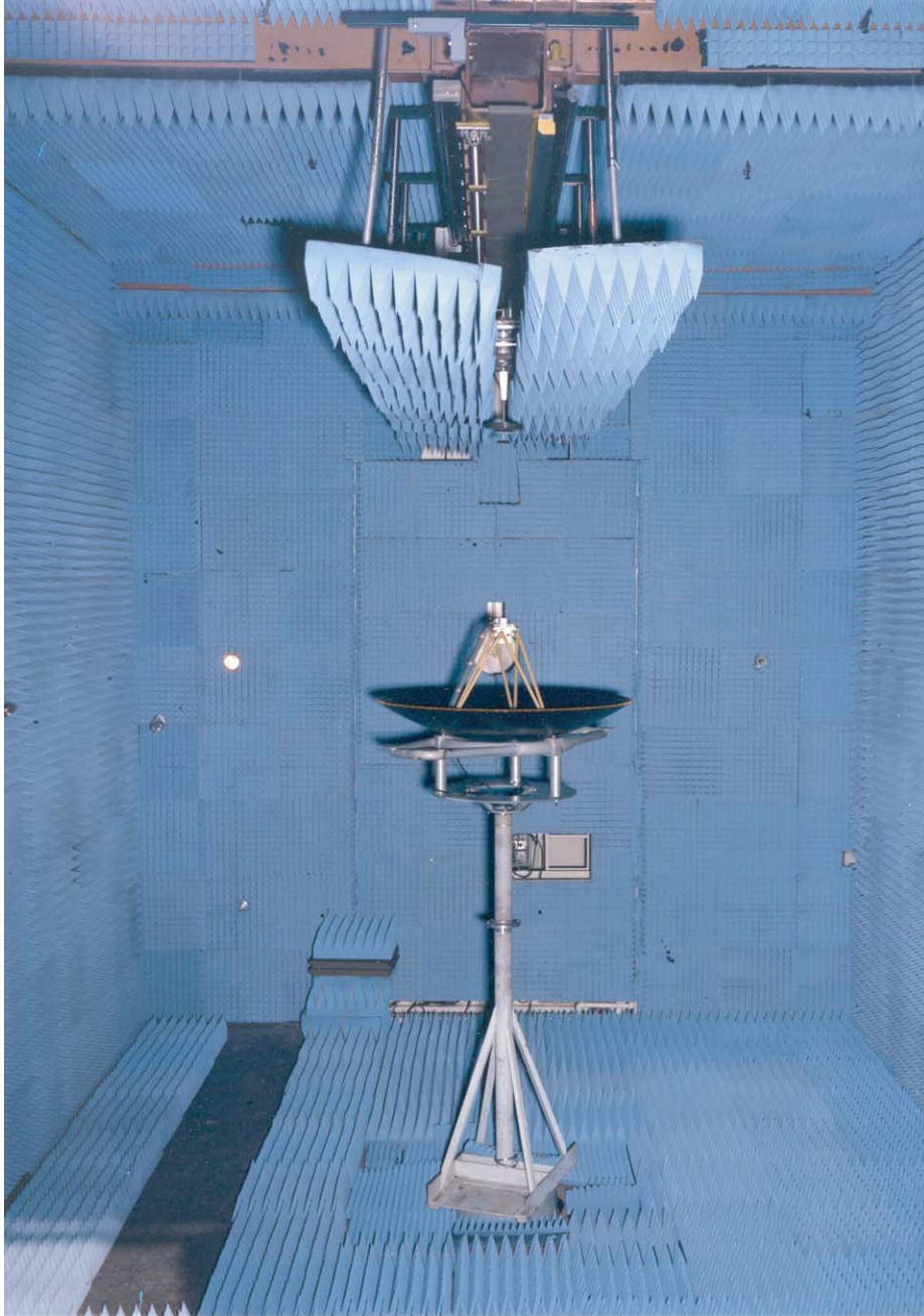
Fig. 1-38. Viking spacecraft HGA in the near-field facility.
