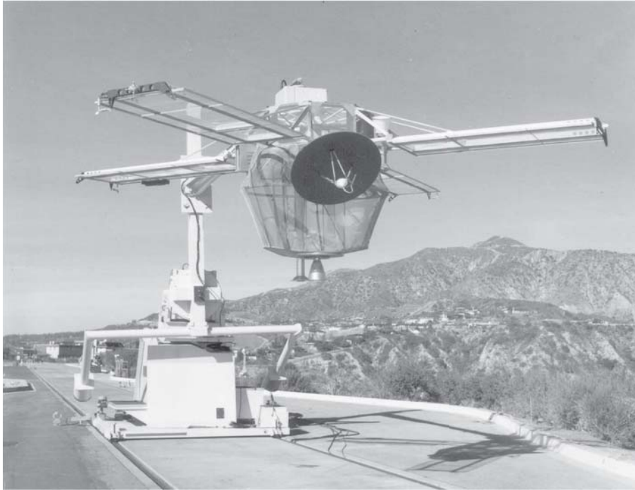
Fig. 4-4. Mariner 9 HGA with spacecraft mockup at the Jet Propulsion Laboratory (JPL) Mesa Antenna Range.
