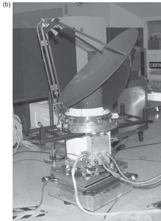
Fig. 7-20 (a) SeaWinds conical-scan spot-beam scan pattern and (b) 1.07 m x 0.96 m Ku-band SeaWinds dual-feed reflector antenna. The reflector shell, waveguides, and feeds are made of lightweight composite material (total weight is 6.40 kg).
