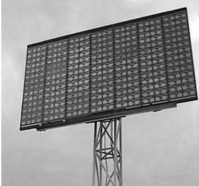
Fig. 10-15. Photograph of the half-size thin-membrane array with seven foldable panels, shown on a test fixture at an outdoor far-field range.
