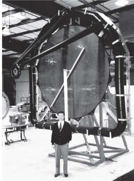
Fig. 10-5. Inflatable Ka-band 3-m reflectarray antenna. The white-colored structure in front of the aperture is a membrane-flatness measurement device.
