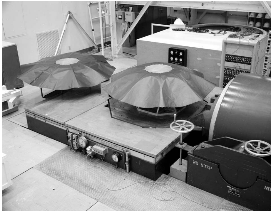
Fig. 5-11. Galileo tip sunshield being tested on the lateral vibration fixture.
