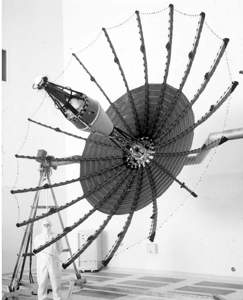
Fig. 5-14. Galileo antenna deployed on its ground handling fixture.
