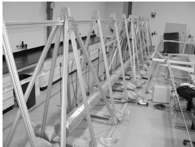
Fig. 10-14. 10-m inflatable boom and its support structure for vibration test.
