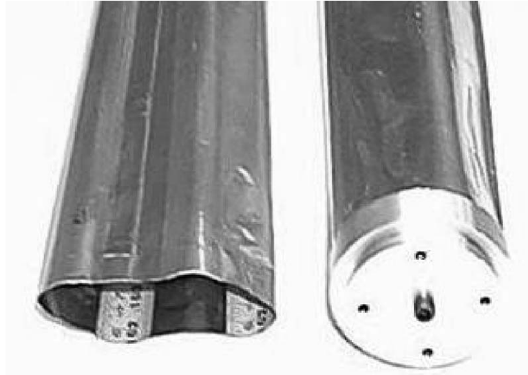
Fig. 10-10. Rigidizable inflatable aluminum tubes reinforced by carpenter tapes. Right tube shows the end cap.
