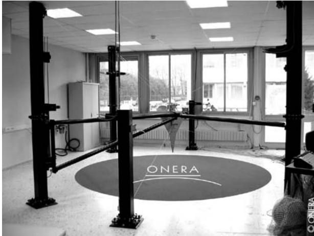
Figure 2.67. The SACSO wire robot for testing a plane model in a wind tunnel (copyright Onera).
