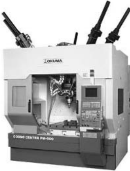
Figure 2.91. The Okuma 5-axis Cosmo Center PM-600 and a detail of its head (courtesy Okuma)
