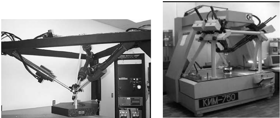
Figure 2.99. On the left, the measuring machine HCCM developed by the University of Florida and Perry Automation □ PA with 5 actuated legs and a passive one. A laser interferometry system allows to measure the leg lengths (courtesy Perry Automation). On the right, the KIM 750 measuring machine of Lopic company, Russia □ LA
