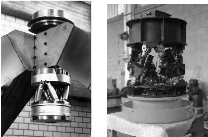
Figure 2.70. Hexapod used for secondary mirror alignment: on the left at the United Kingdom Infra-Red Telescope (UKIRT) and on the right at the Telescopio Nazionale Galileo (courtesy ADS International □ ADS )
