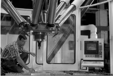
Figure 2.90. On the left, the Octahedral Hexapod of Ingersoll (photo by Kathie Koenig Simon/NIST). On the right, the 6X (courtesy Mikromat)
