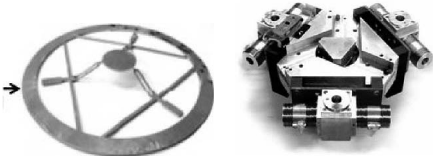
Figure 2.62. The HexFlex 6 d.o.f. robot for micro-positioning. The planar compliant mechanism on the left is deformed by 6 magnetic actuators, 3 in the mechanism plane and 3 perpendicular to the plane
