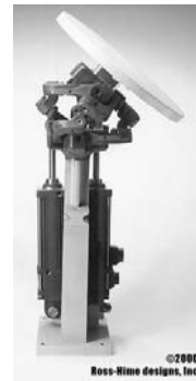
Figure 2.15. On the left, the 3\text{-URU} Dymo mechanism. On the right the 2 d.o.f. Omni-Wrist : a clever arrangement of the passive joints and the use of two linear actuators allows for a \pm 90 degrees rotation ability without singularity (courtesy Ross-Hime Designs)
