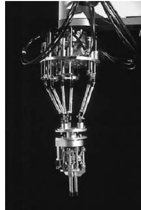
Figure 2.34. The 6 degrees of freedom active wrist , the joints of which that are near the base move vertically, using a chain of the PUS type (INRIA patent).
