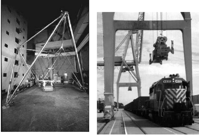
Figure 2.64. On the left, the NIST Robocrane (courtesy NIST). On the right, the DARTS system (courtesy August Design)
